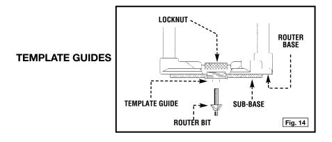
A wide variety of template guides is available for use in pattern and templet routing operations. A typical combination bit, template guide, and locknut are illustrated in Fig. 14.
